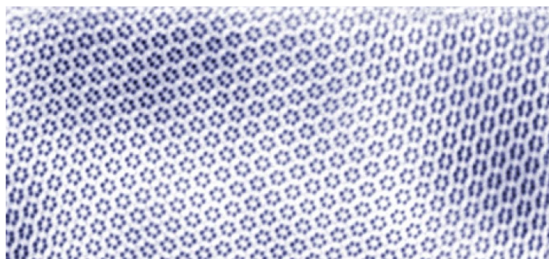
Atomic resolution image of hydrogen-storing metal hydrides. (HZG/Div. Metal Physics)
