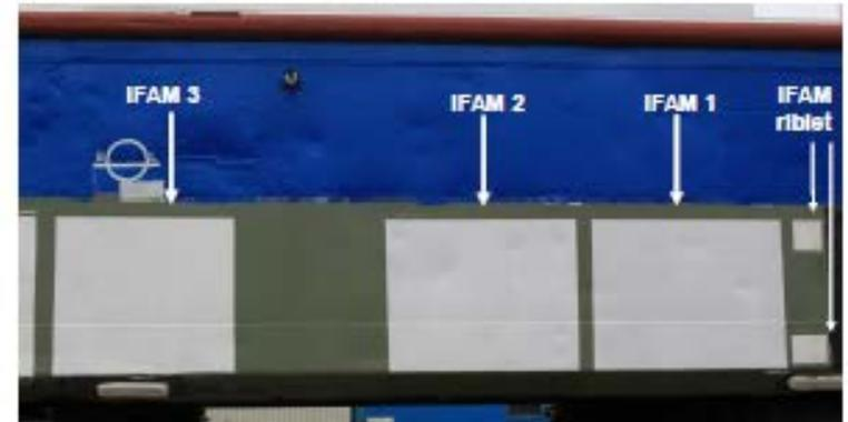
3x 1 m<sup>2</sup> test fields and two riblet fields
